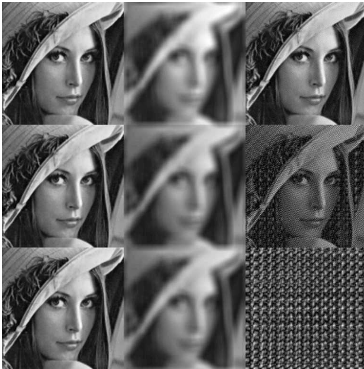
Figure 1: Inverse filtering: Convolution by a 9 \times 9 flat kernel L and addition of uniform noise u (SNR 86, 66, and 46 dB). Left: original x ; center: degraded y = Lx + u ; right: restored. Even though the noise level is low, the performance is very poor.
