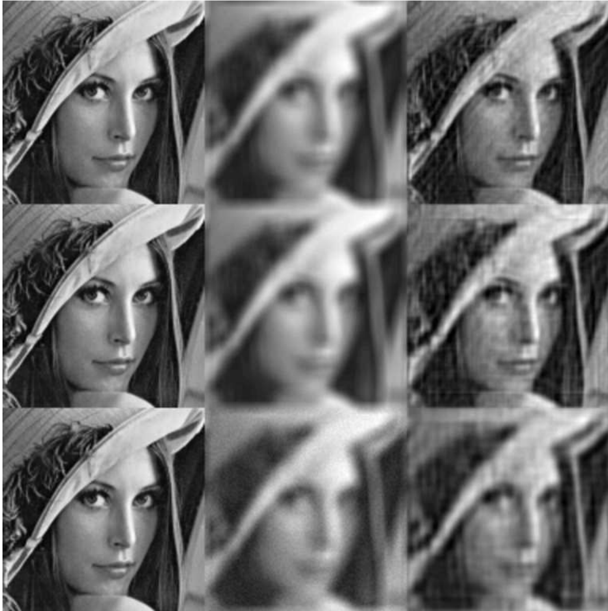
Figure 3: Wiener filtering: Convolution by a 9 \times 9 flat kernel L and addition of uniform noise u (SNR 65, 45, and 23 dB). Left: original x ; center: degraded y = Lx + u ; right: restored. Even though the noise level is higher than in Fig. 1, the results are better, although the edges are very smooth.
